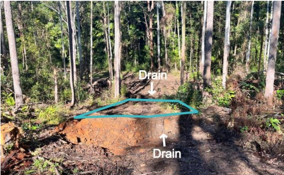
Figure 2-5 Image of a track with the ‘contributing track area’ described in Equation 1 outlined in blue.
