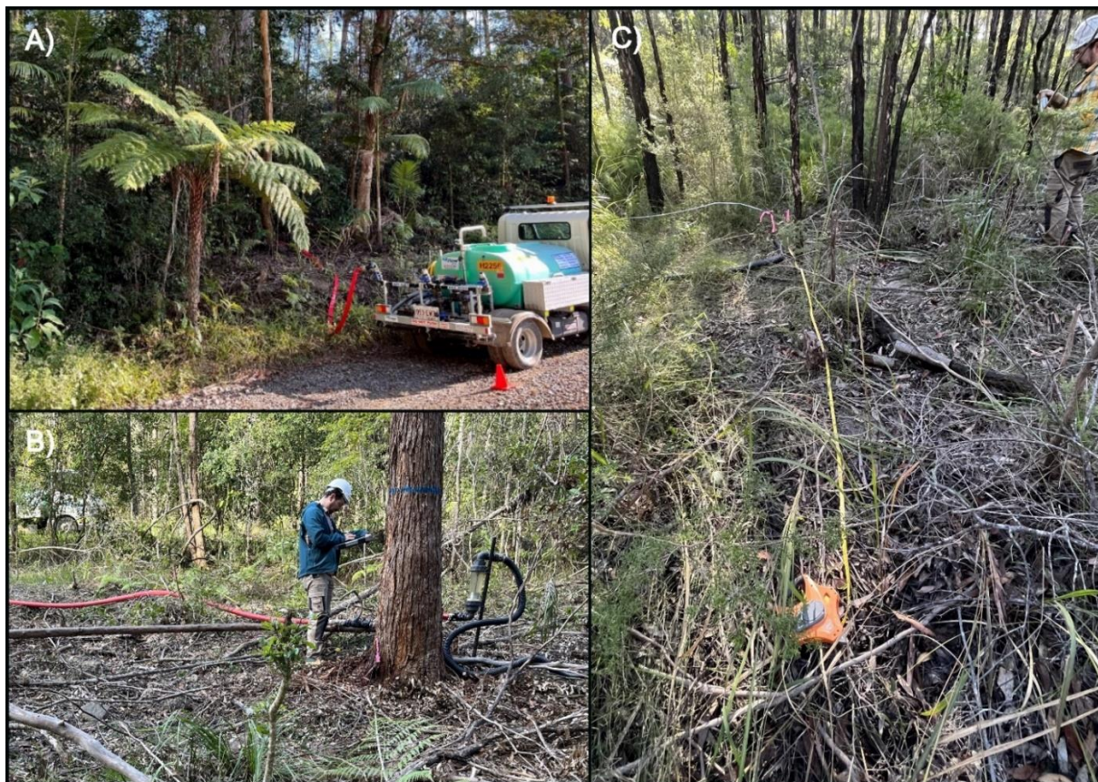
Figure 2-3 General setup of the volume-to-breakthrough experiment. A) depicts the water cart with the water pump attached to the back with the red hose leading into the buffer zone; B) shows the red hose connecting to the rotameter which controls the flow released through the black hose; C) shows the black hose laid out at the top of a vbt5 run (marked by pink tape) with the measuring tape indicating the distance from the discharge point.
